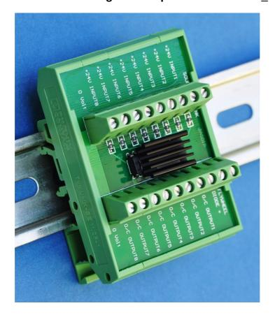
When connecting different manufacturer's equipment together it is sometimes necessary to convert sourcing outputs to sinking. The board uses an ULN2804 IC as a driver. Specifications are as per a ULN2804A.
